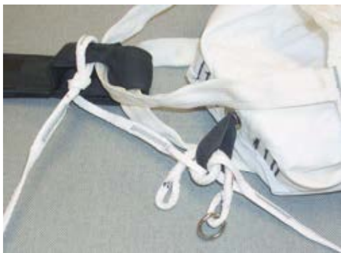
Pass the soft link through the three loops a second time.
