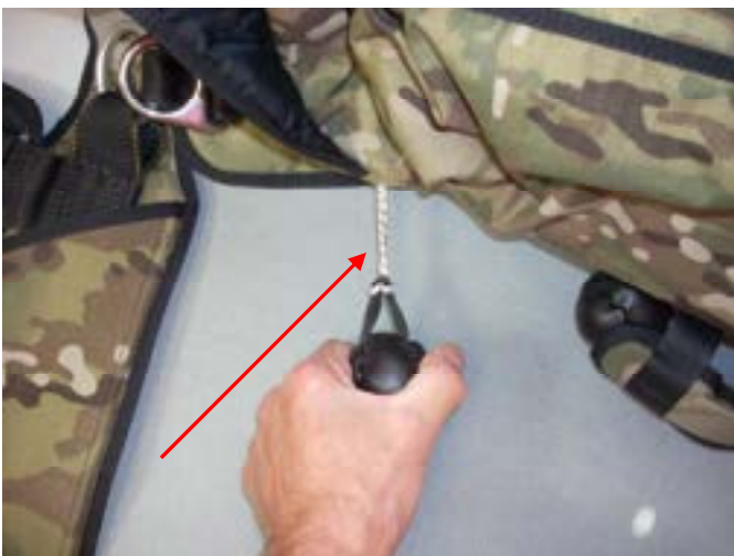
The left side release lanyard removed.
