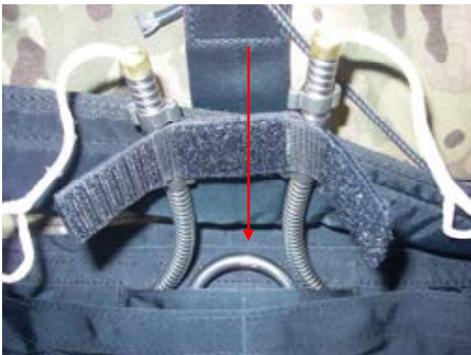
Note the large ring of the internal lateral/diagonal harness used to attach the drogue 3-ring riser.
