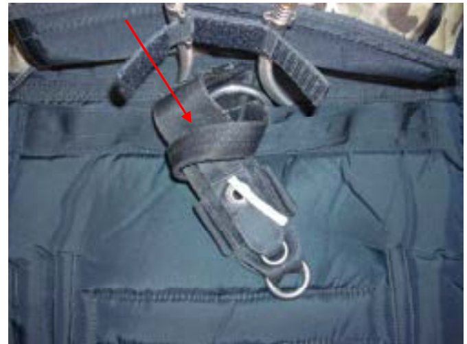
Pass the 3-Ring riser through the loop on the end of the riser.
