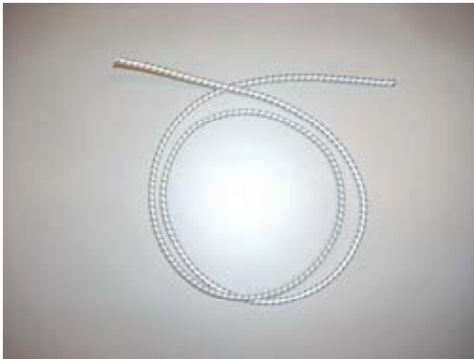
Pictured above is the replaceable drogue release pin elastic.
