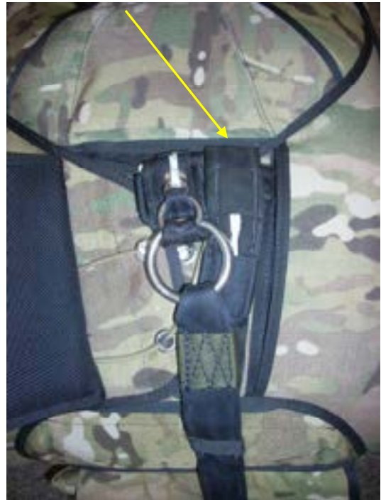
Tuck the drogue bridle under the top right side flap.
