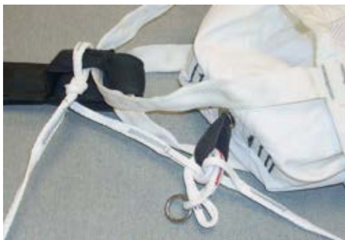
Pass the tail end of the soft link through the end loop beneath the soft link mini ring.
