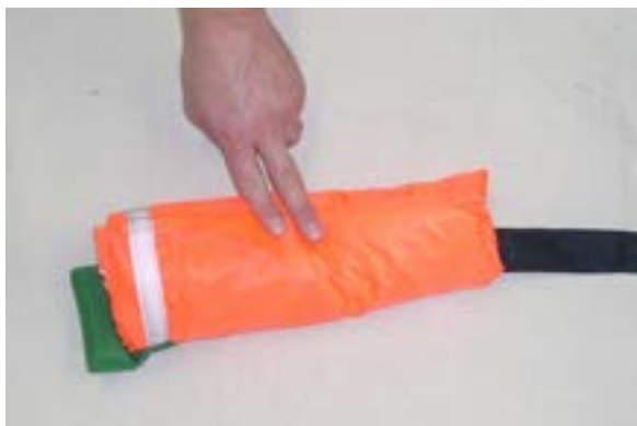
Fold the drogue over the “S”-folded bridle.
