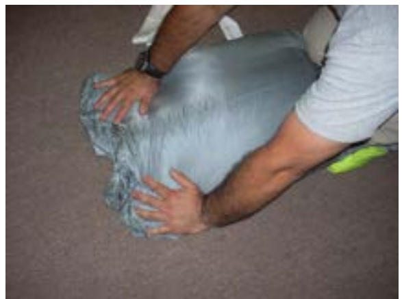
Smooth out and make sure that the canopy is no wider than the free-bag.
