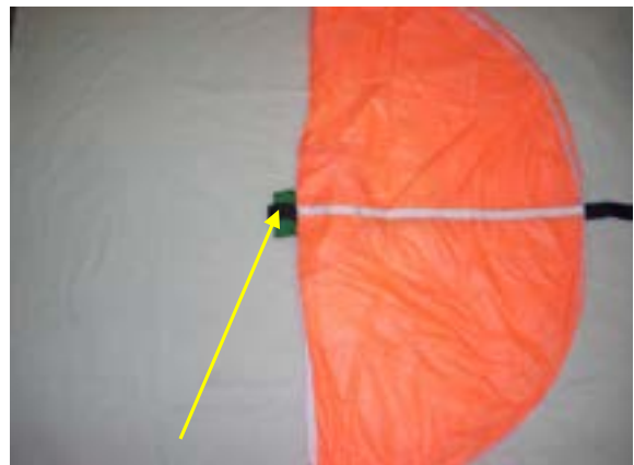
Fold the drogue in half with the bridle exiting the bottom of the curved side and the magnet facing up.
