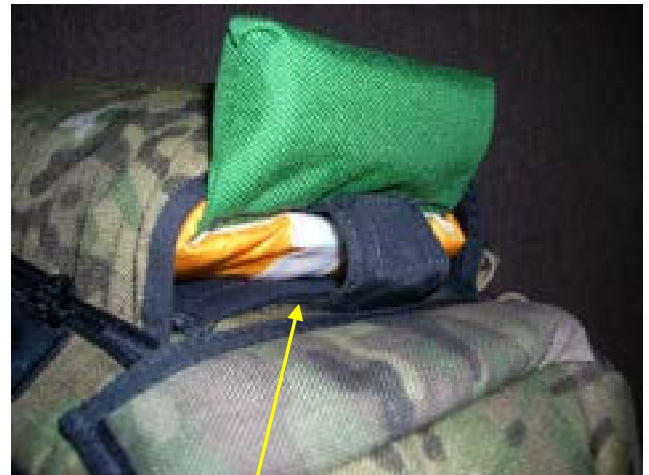
Tuck the T-III tab w/magnet into the pocket of the drogue pouch.
