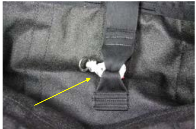
Twist the soft link so that the stainless steel mini ring is exposed from under the loop of the deployment bag.
