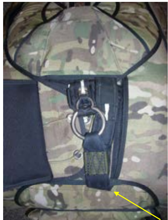
Tuck the drogue bridle under the bottom of the right side flap.
