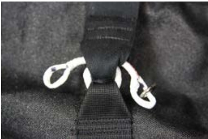
Pass the soft link twice through the loops.
