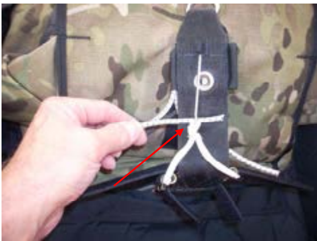
Remove the elastic from the straight pin.
