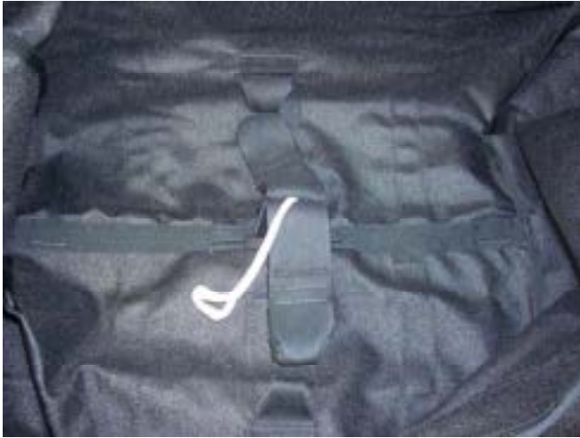
The drogue bridle through the slot on the bottom of the deployment bag.
