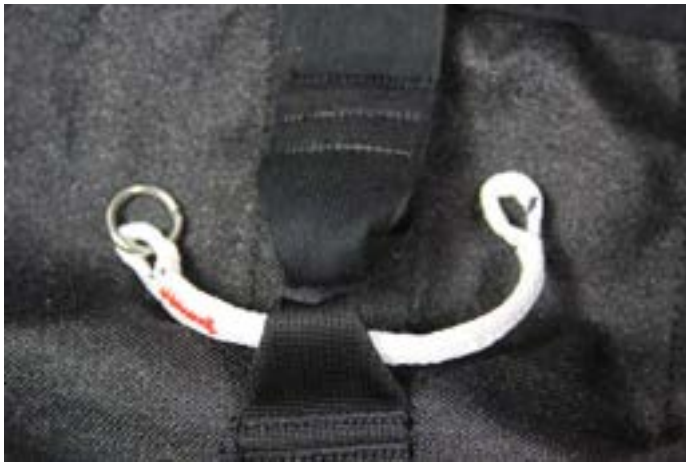
With the drogue bridle inserted into the deployment bag, pass a soft link between the loop of the deployment bag and the loop of the drogue bridle .
